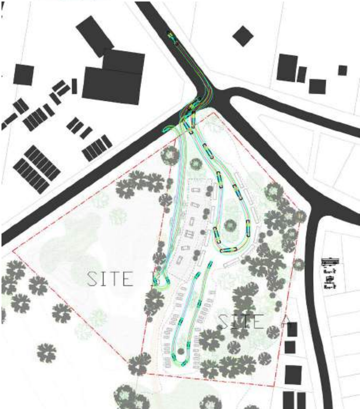
Figure 7: Swept Path Analysis (design drawings version 16-05-2018)
