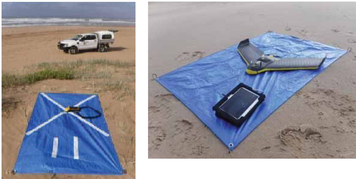
Figure 4 Left: Differential GPS survey of GCPs. Right: eBee Sensefly with operator controller.
